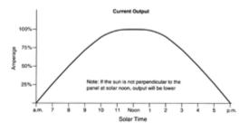
Allowing for recharging inefficiencies, this is still about 50% more than necessary to float a 100-amp-hour battery. A good rule of thumb is 3.5 watts per 100 amp-hours of battery capacity. But throw in an occasional sunless day, put blocking diodes in the circuit, and let the bilge pump run once in a while, and five watts will be about right. A small amount of extra capacity won't damage the batteries as long as you maintain the water level in them.
